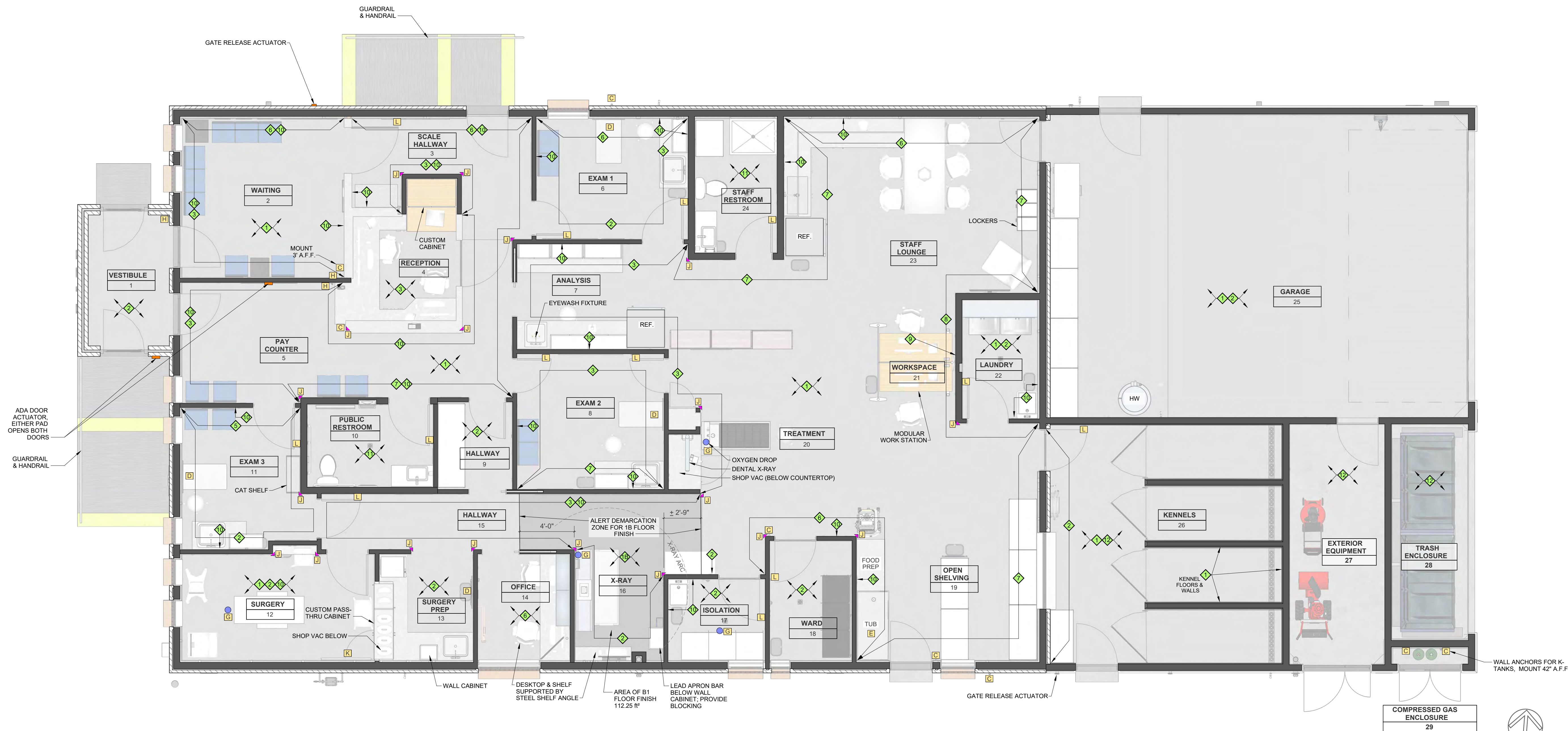
WALL ANCHOR (TRX OR EQUAL) PROVIDE REINFORCED BLOCKING FOR EACH LOCATION MOUNTED 24" A.F.F., U.N.O. (8 TOTAL) SYMBOL 2
