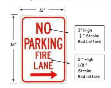
Fire Lane Sign Characteristics: Signs shall be engineer grade reflective sheeting on 0.80 aluminum with red lettering on a white background.
