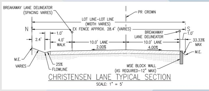
• The reflective vertical delineator which is flexible or breakaway serves as a visual and physical lane delineation between travel lane and pedestrian path . This is to solve the safety concerns raised by the citizens.
