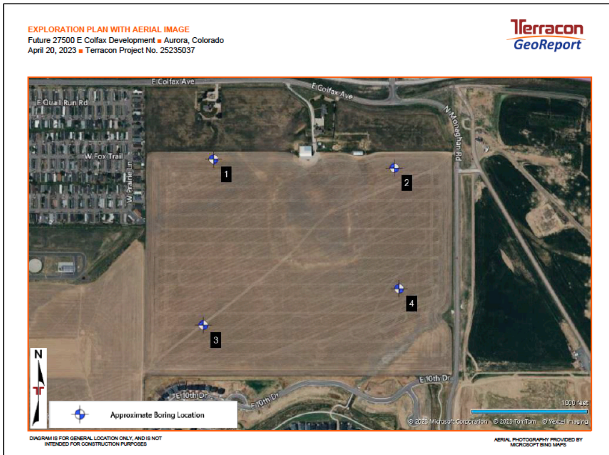
Boring Holes Drilled
