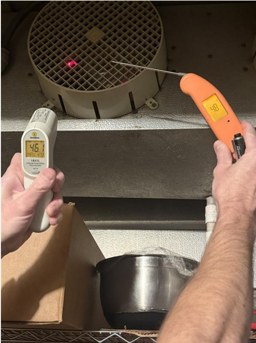
May 15, 2026: Inspector thermometers showing walk-in refrigerator holding temperature at 48F.
