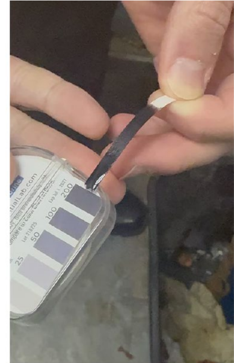
May 1, 2026: Sanitizer used for dishes during cleaning at toxic levels.
