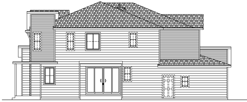
9 RIGHT ELEVATION B - D770 W/ OPT. BR3 @ D769 SCALE: 1/8"=1'-0" FRONT ELEVATION DOES NOT CHANGE WITH THIS OPTION RE: 1/A22 FOR ADDITIONAL NOTES & DIMENSIONS
