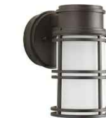
WL1 - Wall mount at Trellis Entrances, 8 Watts, 3000 Kelvin, Bronze Painted, Mount at ADA Height
