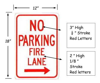
**Fire Lane Sign Characteristics:** Signs shall be engineer grade reflective sheeting on 0.80 aluminum with red lettering on a white background.
